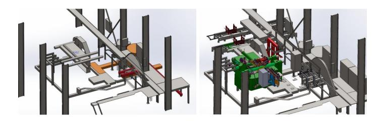
Erie then designed the new platforms to support the equipment and crossovers and guardrails to allow access and protect personnel:
